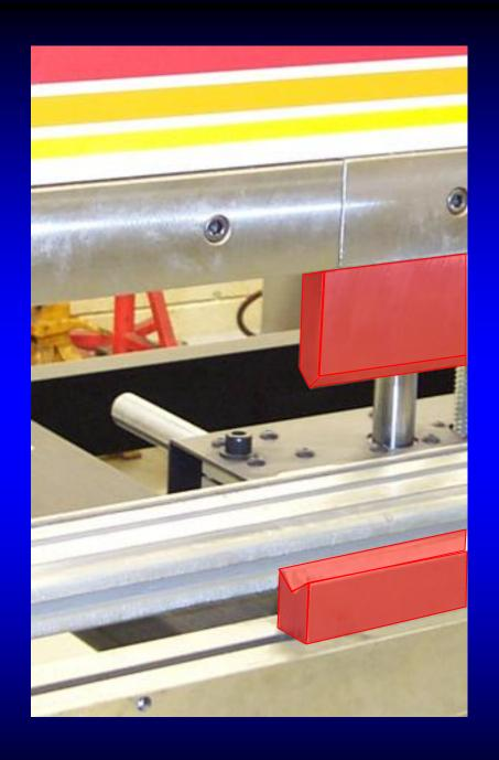
As with all sheet metal tools, the brake presents a significant hazard where the tool meets the work. Keep hands away from the working area.
