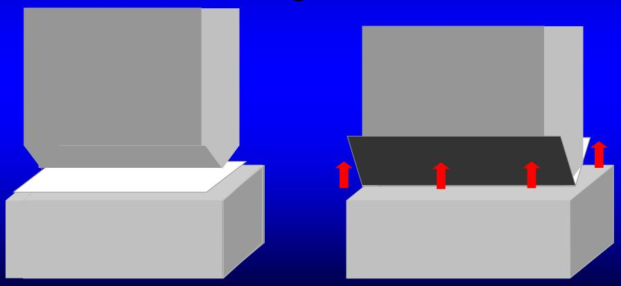
After operating the sheet metal brake, make sure the ram is set at the bottom of its stroke and the power is turned off.
