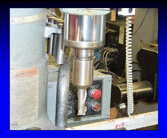
Cutters should be keyed to the arbor and run in the correct direction to give the proper "up" or "down" milling desired.
