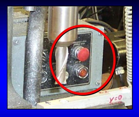
If you are changing arbors, cutters or making any adjustments or changes in the setup, turn the power off.
