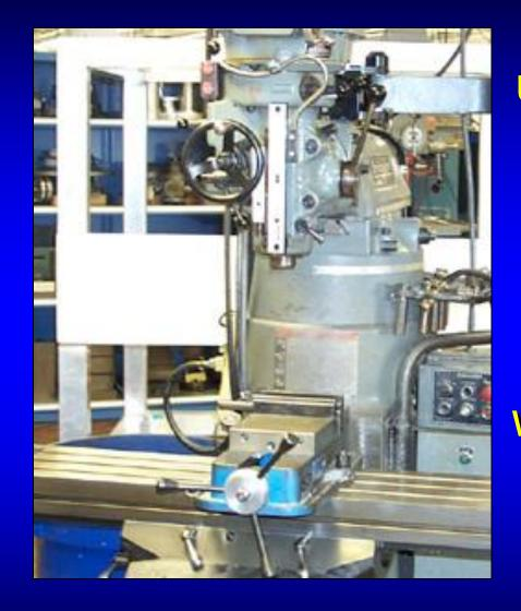
A milling machine is used to machine flat or irregular surfaces. It can also be used to drill, bore, cut gears, and produce slots. It removes metal from a workpiece by rotating a multi-toothed cutter that is fed into the moving workpiece.
