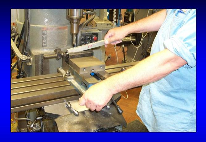
Before running the machine it should be tried manually to make sure it is clear for cutting.
