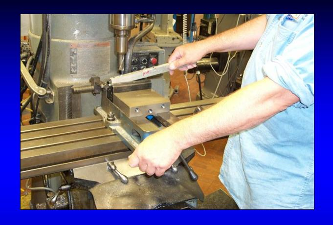
When operating the milling machine, be sure hands are properly placed away from the cutting tool.
