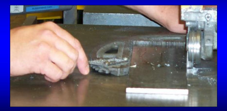
Or, if you need to cut completely through a workpiece, you can guide it using a block of wood.
