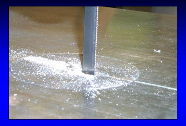
The band saw is used for cutting stock to size and roughing shapes. It contains a serrated blade that runs between two pulleys.
