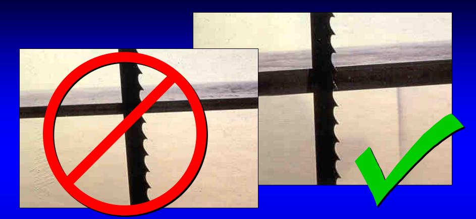
Use the proper blade for the material. The material to be cut should be at least two tooth widths in thickness. Also, never use a soft metal blade to cut hardened material.
