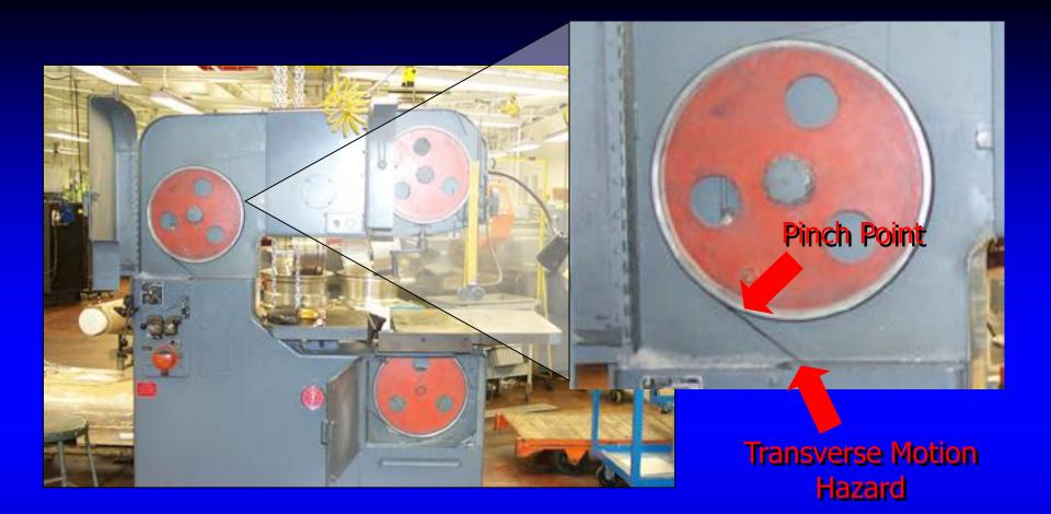
When left unguarded, exposed pulleys and blades present a hazard where the moving band can pull loose objects into pinch points.
