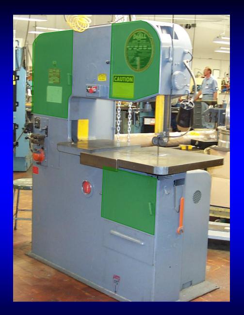
Make sure the pulleys that propel the band saw are guarded while in motion.
