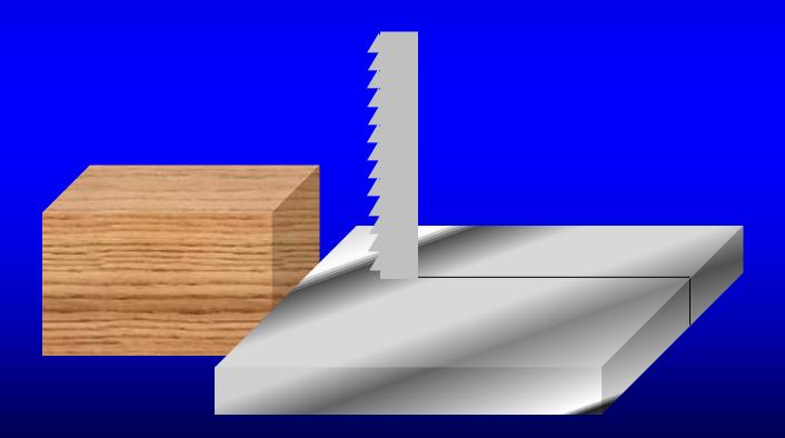
Before starting the band saw, adjust the blade guard to the appropriate height. Always set the blade guard just high enough to clear the part you're cutting. The less blade exposed, the safer it is.
