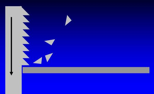
Cutting improper material or cutting with an improper blade can result in a serious hazard. The serrated teeth of the blade can snap off on contact with the material.
