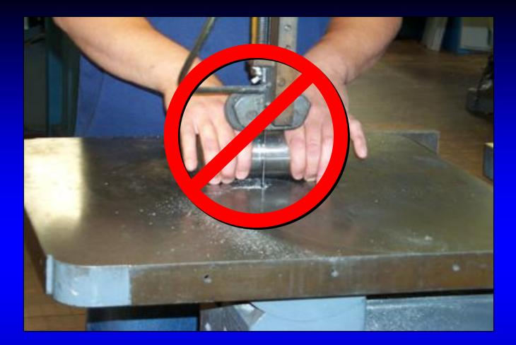
Never cut round stock in a band saw! The serrated blade can catch the workpiece and present a serious hazard.
